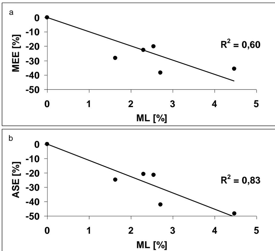
**Fig. 3.** Moisture exclusion efficiency (MEE) (a) and anti-swelling efficiency (ASE) (b) vs. mass loss (ML)
