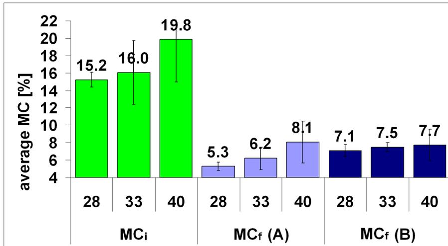
Fig. 1. Average and standard deviation for the initial and final MC at different thickness values
