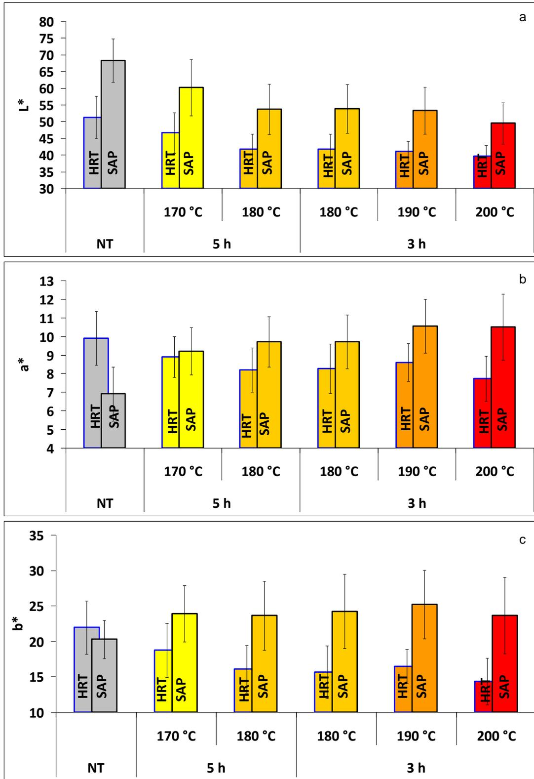
Fig. 5. Colour coordinates  $L^*$  (a),  $a^*$ (b), and  $b^*$ (c) of sapwood and heartwood of untreated and treated wood at different process conditions.
