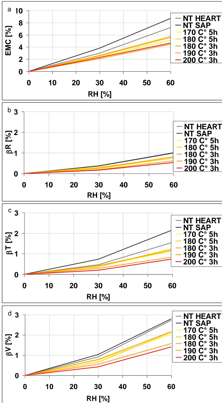
**Fig. 4.** Equilibrium moisture content EMC (a), radial  $\beta_R$  (b), tangential  $\beta_T$  (c), and volumetric swelling  $\beta_V$ (d) vs. RH
