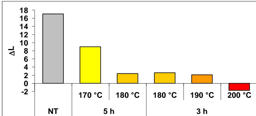
**Fig. 6.** Lightness difference ( $\Delta L$ ) between treated sapwood and untreated heartwood (sapHT - heartNT)
