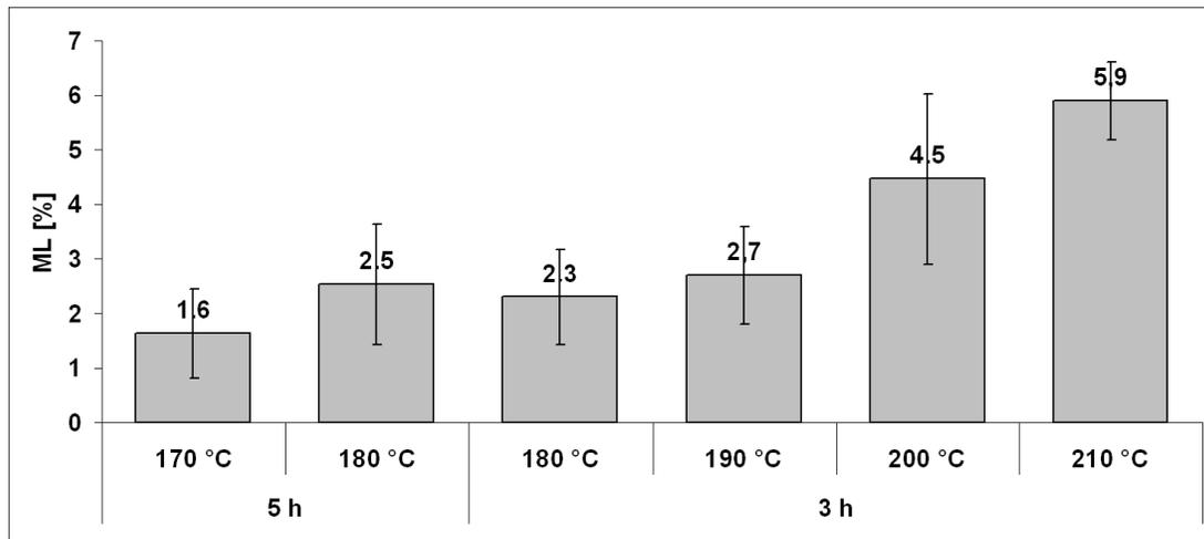
Fig. 2. The mass loss (ML) measured for the tested processes
